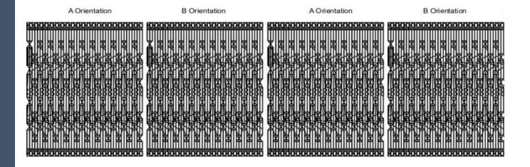
NOTE: Packs with an odd number of sheets will have short flutes on top section of both sides and long flutes on bottom. To prevent these packs from nesting, install one pack with short flute up and next pack with short flute down. This "flipping" method will insure a proper orientation as illustrated above, (short flute next to long flute).
